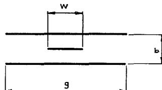
Fig. 1. Strip transmission line.
